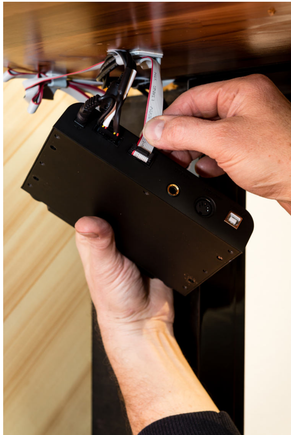
fig. 3.1: Wiring of communication cables of keyboard and pedal
