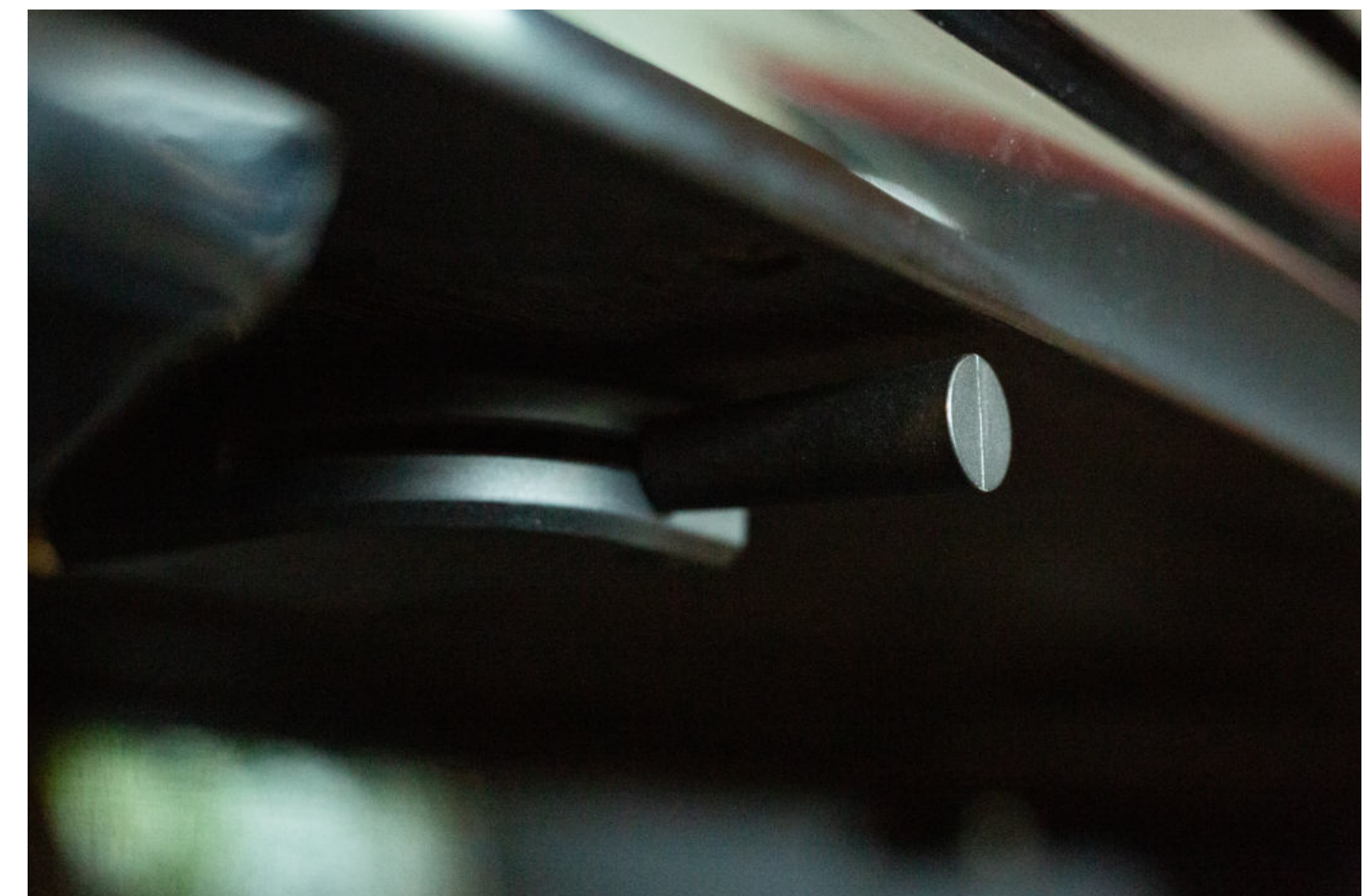
fig. 1.25: The mute lever is flush with the front of the piano when pulled
