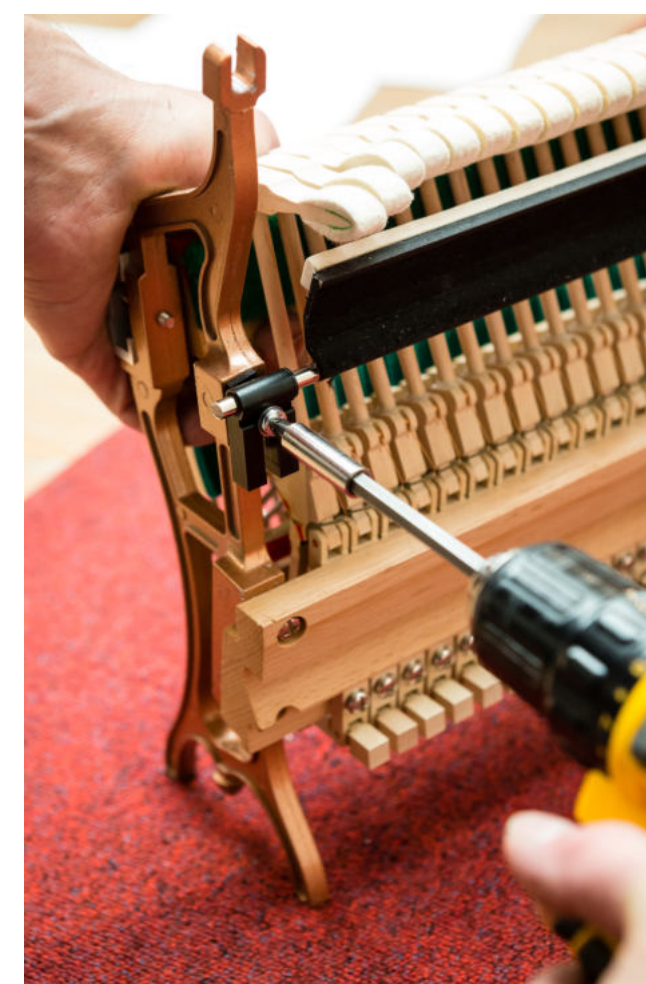
fig. 1.16: Height check: Hammers cannot touch the mute rail.
