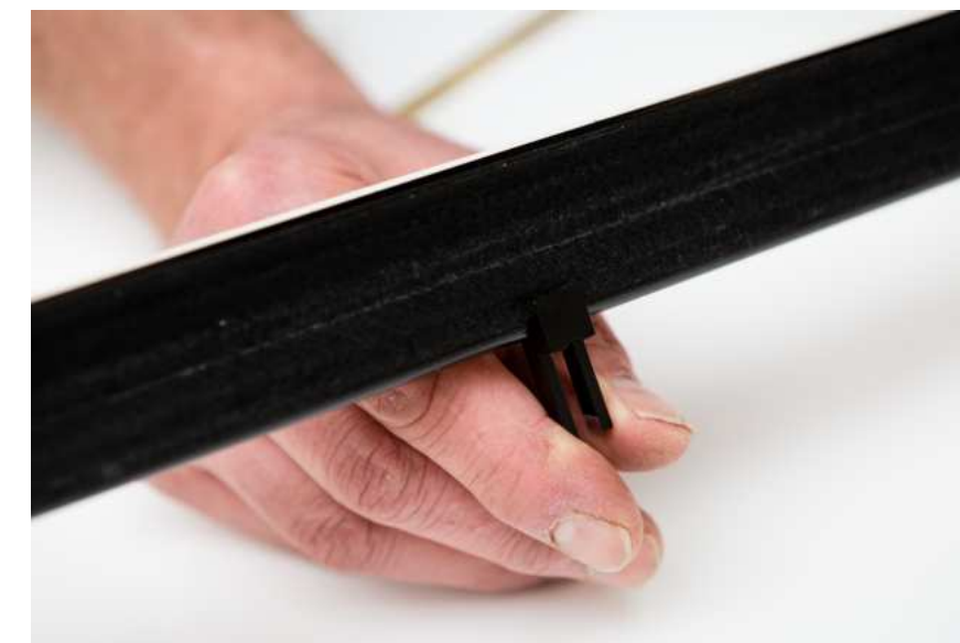
fig. 1.2: Position the bracket in the middle of the mute rail
